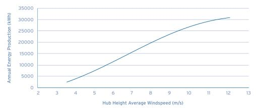
The AEP Curve (Annual Energy Production) demonstrates the energy the KW6 will generate on sites with a given average wind speed at hub height. The ability to calculate kWh / year allows for clear estimations of financial viability to be calculated.
